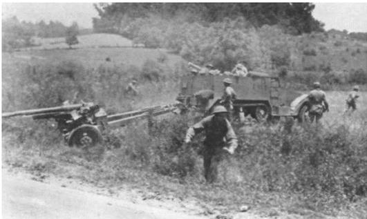
3 inch M5 anti-tank gun towed by a half-track
